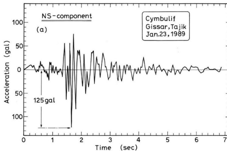
**Figure 6. Strong motion record of the Hissar earthquake, distance from the epicenter about 5 km
